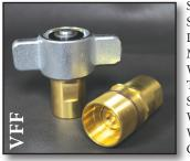
Screw to Connect Locking: Screw Together Material: Brass Body Wing Nut: Carbon Steel hreads: NPT tandard Seals: NBR Working Temperature: -13°F +212°F Working Pressure: 2,500-3,000 PSI Connect under pressure: **Not Suggested**
