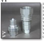
nterchange: Faster VV Screw type Push/Pull Locking: Screw Together Poppet Material: Carbon Steel inishing: Zn-Fe (CR111) hreads: **NPT, BSP** tandard Seals: NBR Working Temperature: -13°F +212°F Working Pressure: 3,350-5,100 PSI Connect under pressure: Not Suggested
