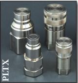
andard: **ISO 16028** Push to Connect Locking: Radial Balls Material: 316 Stainless Steel hreads: **NPT, BSP, SAE** ndard Seals: NBR Working Pressure: **4,200-7,000 PSI** onnect under pressure: **Not Allowed**
