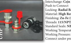
Push to Connect Locking: Radial Balls Material: High Resistance Steel ishing: **Zn-Fe** (**CR111**) reads: 115/NPT, 116/BSP ndard Seals: NBR Vorking Temperature: -13°F +212°F Working Pressure: 15,000-20,000 PSI Connect under pressure: Not Allowed
