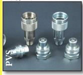
nterchange: With Main Producers Screw to Connect Ball Locking: Screw Together Material: High Resistance Steel Finishing: **Zn-Fe** (**CR111**) hreads: NPT, BSP andard Seals: NBR Working Temperature: -13°F +212°F Working Pressure: 10,290 PSI Connect under pressure: **Not Suggested**
