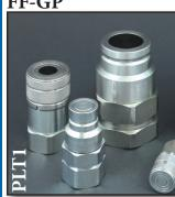
andard: **ISO 16028** Push to Connect Locking: Radial Balls Material: Carbon Steel inishing: Zn-Fe (CR111) hreads: NPT, BSP, SAE ndard Seals: NBR orking Temperature: -13°F +212°F Working Pressure: **3,675-4,630 PSI** onnect under pressure: Not Allowed
