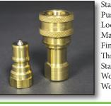
Standard: 7241-B Push to Connect Locking: Radial Balls Material: Carbon Steel Finishing: **Trivalent Chrome Plating** Threads: NPT, SAE Standard Seals: NBR Working Temperature: -13°F +212°F Working Pressure: 6,000 PSI
