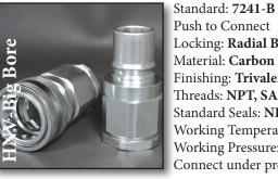
Locking: Radial Balls Material: Carbon Steel Finishing: **Trivalent Chrome Plating** Threads: NPT, SAE Standard Seals: NBR Working Temperature: -13°F +212°F Working Pressure: 6,000 PSI Connect under pressure: **Not Allowed**
