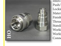
Interchange: Parker Push/Pull Unvalved Locking: Radial Balls Material: 316 Stainless Steel inishing: 316 Stainless Steel Threads: NPT tandard Seals: Buna w/ Teflon Ring Norking Temperature: -13°F +212°F Working Pressure: 10,000-15,000 PSI onnect under pressure: Not Allowed
