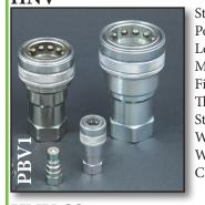
tandard: ISO 7241-B Poppet Style Locking: **Radial balls** Material: Carbon Steel nishing: Zn-Fe (CR111) Threads: NPT, BSP tandard Seals: NBR Working Temperature: -13°F +212°F Working Pressure: 3,675-7,250 PSI Connect under pressure: Not Allowed
