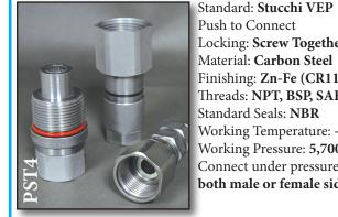
Push to Connect Locking: Screw Together Material: Carbon Steel Finishing: Zn-Fe (CR111)/Zn-Ni Threads: NPT, BSP, SAE Standard Seals: NBR Working Temperature: -13°F +212°F Working Pressure: 5,700-9,000 PSI Connect under pressure: Allowed both male or female side
