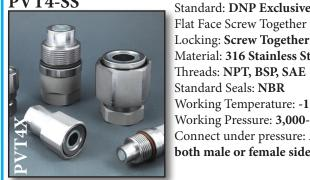
Flat Face Screw Together Locking: Screw Together Material: 316 Stainless Steel Threads: **NPT, BSP, SAE** Standard Seals: NBR Working Temperature: -13°F +392°F Working Pressure: 3,000-5,000 PSI Connect under pressure: Allowed both male or female side
