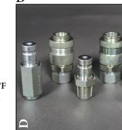
Interchange: With Main Producers Push to Connect Locking: **Radial Balls** Material: Carbon Steel inishing: Trivalent Chrome Plating Threads: NPT, SAE Standard Seals: NBR Working Temperature: -13°F +212°F Working Pressure: **6,000 PSI** Connect under pressure: Not Allowed
