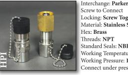
Screw to Connect Locking: Screw Together Poppet Material: Stainless Steel Body Hex: Brass Threads: **NPT** Standard Seals: NBR Working Temperature: -13°F +212°F Working Pressure: 10,000 PSI Connect under pressure: Not Suggested
