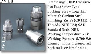
Flat Face Screw Type Locking: Screw Together Material: Carbon Steel Finishing: **Zn-Fe** (**CR111**) - **Zn-Ni** Threads: **NPT, BSP, SAE** Standard Seals: **NBR** Working Temperature: -13°F +212°F Working Pressure: 5,700-9,000 PSI Connect under pressure: Allowed, both male or female side.
