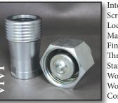
nterchange: DNP Exclusive Screw to Connect ocking: Screw Together Poppet Material: Carbon Steel inishing: **Zn-Fe** (**CR111**) nreads: NPT tandard Seals: NBR Working Temperature: -13°F +212°F Working Pressure: 2,200-3,000 PSI Connect under pressure: Not Suggested
