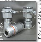
Interchange: **DNP Exclusive** Flat Face Screw Together Locking: **Screw Together w/Pin Lock** Material: Carbon Steel inishing: **Zn-Fe** (**CR111**) Threads: NPT, BSP, SAE Standard Seals: NBR Working Temperature: -13°F +212°F Working Pressure: 5,700-9,000 PSI Connect under pressure: Allowed both male or female side
