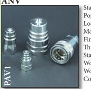
Standard: ISO 7241-A Poppet Style Locking: Radial balls Material: Carbon Steel inishing: Zn-Fe (CR111 Threads: **NPT, BSP, SAE** tandard Seals: NBR Working Temperature: -13°F +212°F Working Pressure: 3,000-5,145 PSI Connect under pressure: Not Allowed
