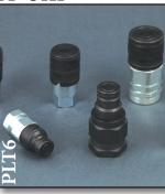
tandard: **ISO 16028** Push to Connect Locking: Radial Balls Material: High Resistance Steel Finishing: Zn-Fe (CR111)/Zn-Ni Threads: NPT, BSP, SAE Standard Seals: **NBR** Working Temperature: -13°F +212°F Working Pressure: 10,000 PSI Connect under pressure: Not Allowed
