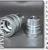
Interchange: Nordic Interchange Decompression Valve Locking: Radial Balls Material: Carbon Steel Finishing: Zn-Fe (CR111) Threads: NPT, BSP Standard Seals: NBR Working Temperature: -13°F +212°F Working Pressure: 4,350-5,000 PSI Connect under pressure: PT: Not Allowed PTK: Allowed both male or
