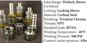
Locking: Locking Sleeve Material: Carbon Steel Finishing: Trivalent Chrome Plating Threads: NPT Standard Seals: BUNA Working Temperature: -40°F +250°F Working Pressure: 500 PSI Connect under pressure: Allowed
