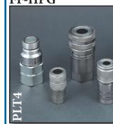
standard: ISO 16028 Push to Connect Locking: Radial Balls Material: Carbon Steel inishing: Threads: NPT, BSP, SAE, JIC, ORFS tandard Seals: NBR Working Temperature: -13°F +212°F Working Pressure: 6,100-7,350 PSI
