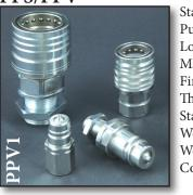
Standard: ISO 7241-1A Push/ Pull Locking: **Radial Balls** Material: Carbon Steel nishing: Zn-Fe (CR111) Threads: NPT, BSP & METRIC Standard Seals: NBR Working Temperature: -13°F +212°F Working Pressure: 2,490-3,675 PSI Connect under pressure: Not Allowed
