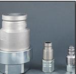
Standard: ISO 16028 Push to Connect Locking: Radial Balls Material: **High Resistance Steel** Finishing: Zn-Fe (CR111)/Zn-Ni Threads: **NPT, BSP** andard Seals: NBR Working Temperature: -13°F +212°F Working Pressure: **6,100-7,350 PSI** Connect under pressure: **Allowed** (male side only) Max Residual Pressure: 250 bar
