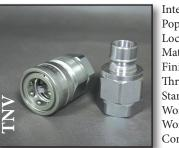
Interchange: General Purpose Poppet Style Locking: Radial Balls Material: Carbon Steel Finishing: **Zn-Fe** (**CR111**) hreads: NPT Standard Seals: NBR Working Temperature: -13°F +212°F Working Pressure: 1,500-6,500 PSI Connect under pressure: Not Allowed
